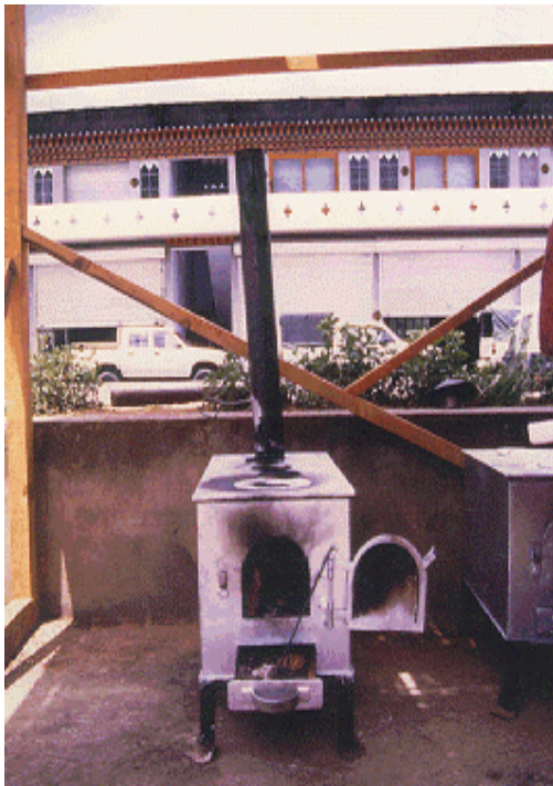
Metallic stove with chimney for combined application of cooking and space heating (TB).
