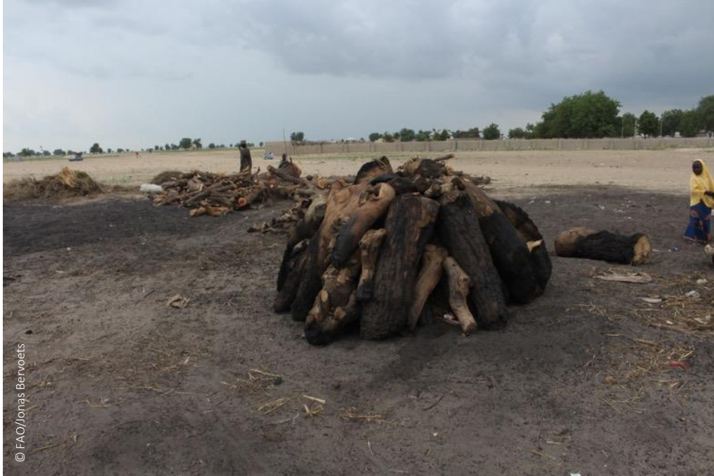
Figure 30 – During the first step of the charcoalization process, burnt wood logs are assembled to form a pyre.
