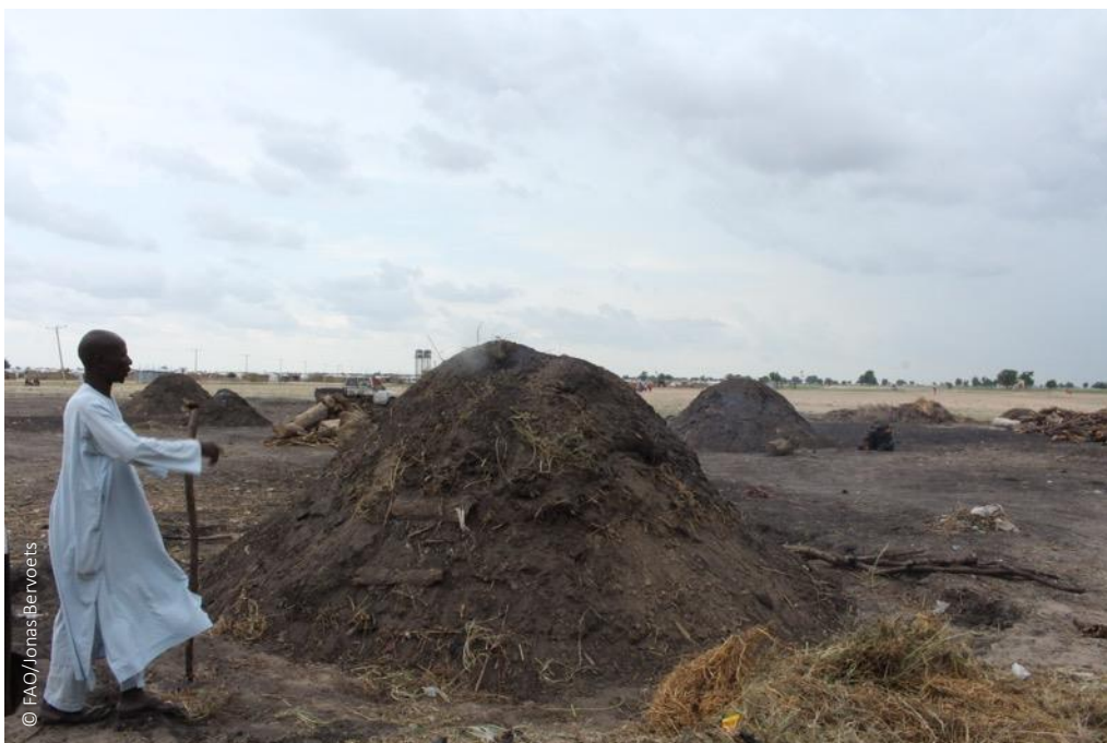
Figure 31 - After lighting, the pyre is covered with soil until the end of the process.
