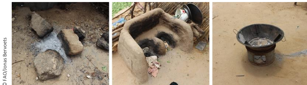
Figure 23 - Most common cooking technologies (left to right: three stones fire, mud stove, metal stove).
