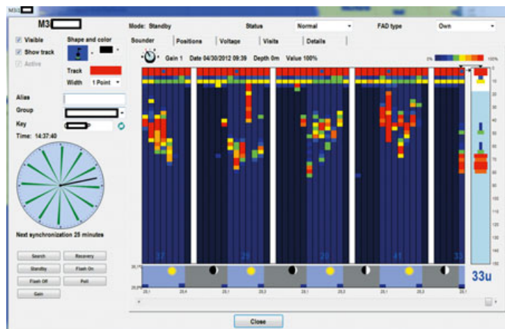
Figure 2 Picture of echosounder readings from the screen of a computer onboard a purse seiner in the Atlantic ocean showing fish biomass underneath a fish aggregating devices (FAD) as observed by an echosounder buoy attached to the FAD (courtesy of Marine Instruments). The image covers 4 days with information provided by the echosounder every 2 h. An aggregation of fish (likely to be tunas) is observed between 20 and 70 m. These data do not allow species discrimination.
