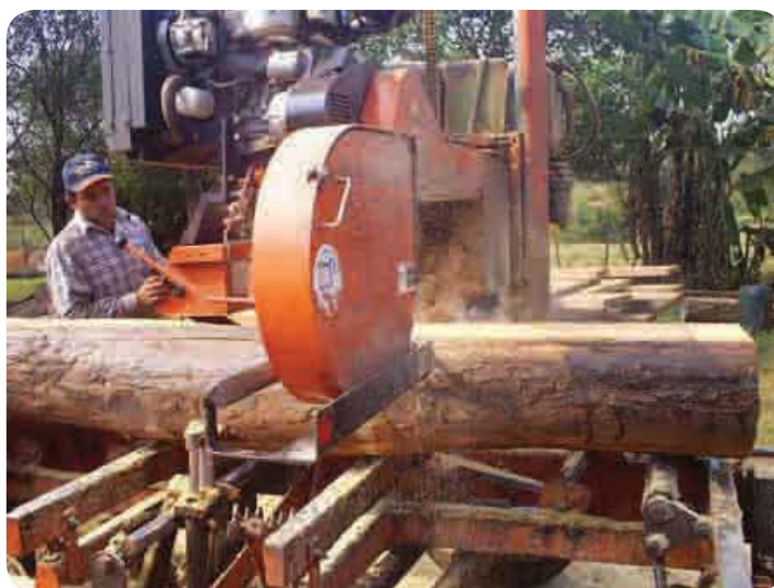
Use of a mobile sawmill to produce planks from logs of timber from the farm of Juan de Dios Ojeda
