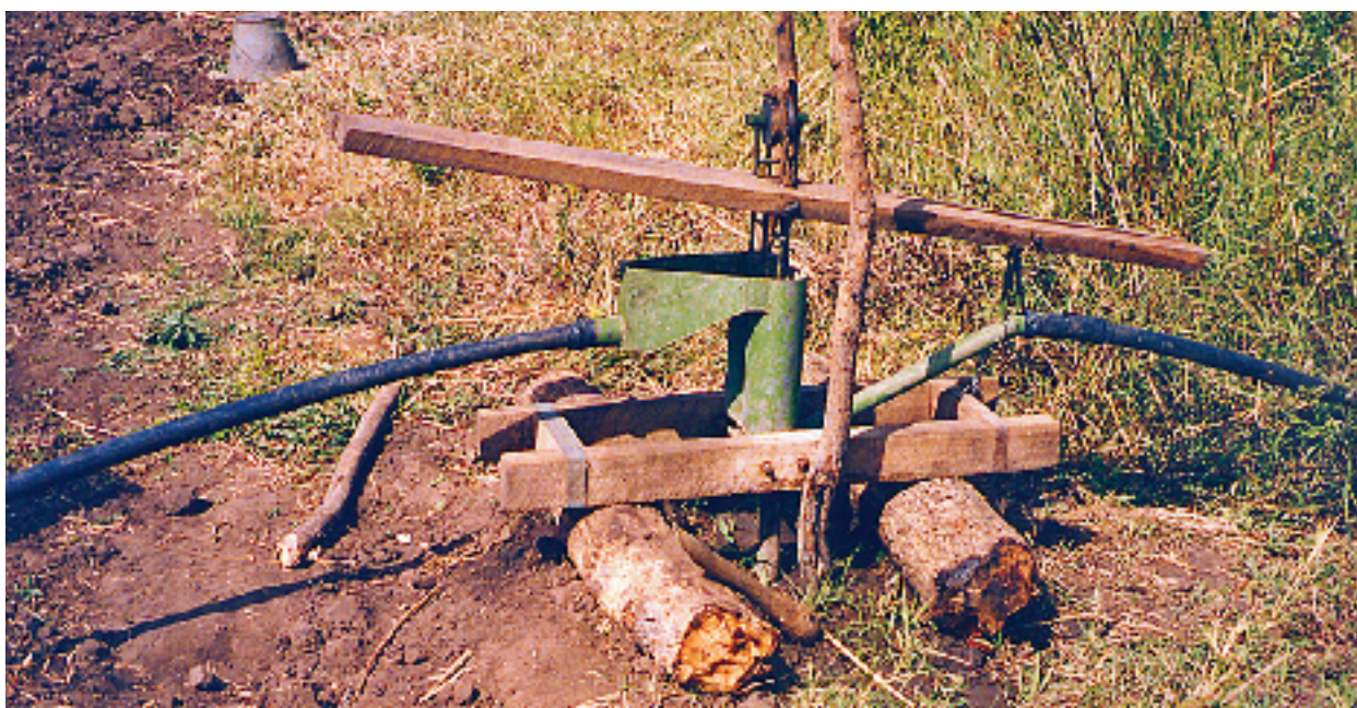
IDE modified river pump, Zambia.
