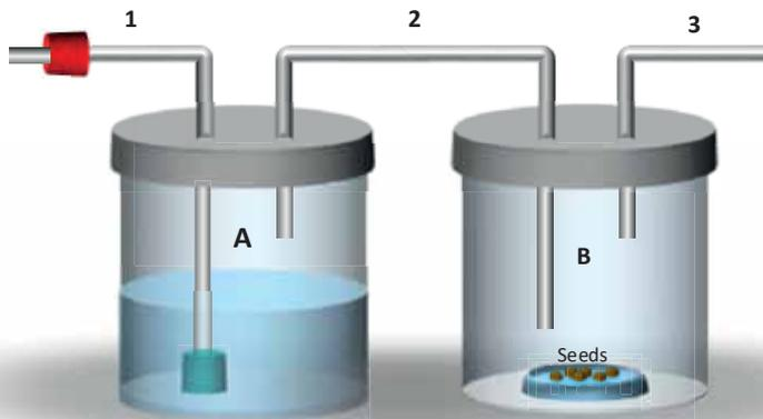
*Figure 1.5. Humidity (water content) adjustment in seeds. The system for adjusting seed moisture (water content) uses flow-through chambers. The gas (or air) to be humidified) flows through tube 1 into the glycerol-water solution in jar A. The humidified gas then flows through tube 2 into the controlled-environment chamber (jar B) and exits into the atmosphere through tube 3. (Modified from Forney and Brandl, 1992).*
