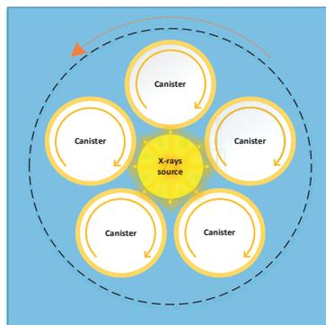
X-ray tube (centre) surrounded by orbiting and rotating sample canisters.
