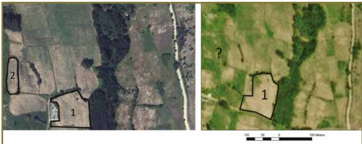
FIGURE 21. PHOTOINTERPRETING PLOTS WITH AN AERIAL ORTHOPHOTOGRAPH (0.5 M RESOLUTION) AND A SATELLITE IMAGE (2.5 M RESOLUTION).
