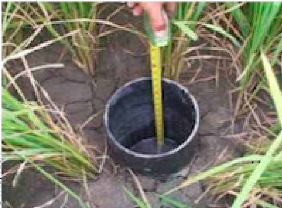
Figure 1. Field water tube from PVC
