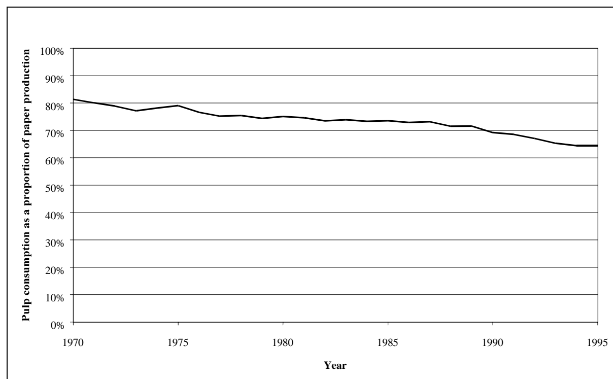
Figure 1: Trend in the utilisation of pulp in the manufacture of paper
