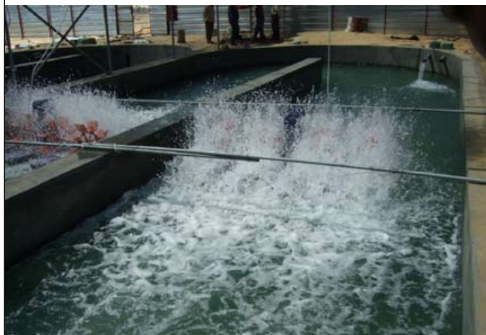
FIGURE 13 D-ended shape European seabass raceway (185 m 3 ) with 2 HP paddlewheel, in Rula land reclamation company, Wadi Group, El-Beheira Governorate, Egypt
