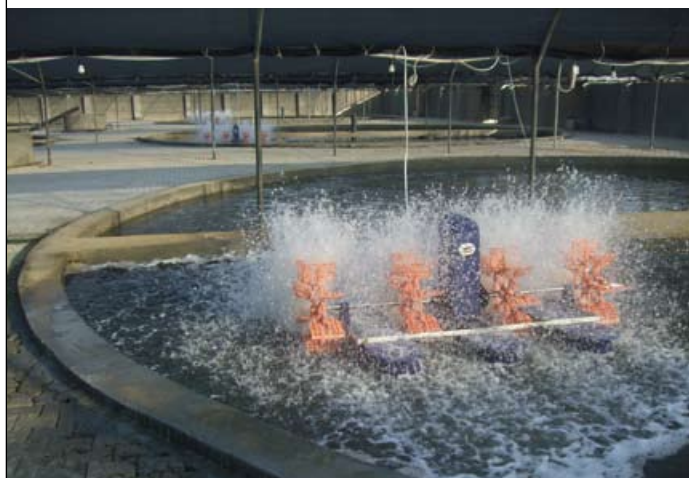
FIGURE 14 European seabass circular tank (340 m 3 ) with 2 HP paddlewheel, in Rula land reclamation company, Wadi Group, El-Beheira Governorate, Egypt
