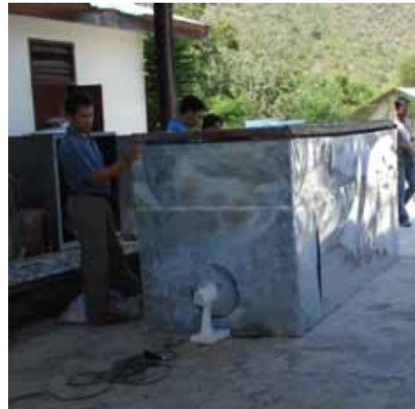
Figure 2. Dryer adapted for anchovy, Indonesia
